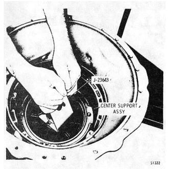
Fig. 5-15. Removing center support assembly
