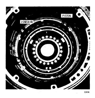
Fig. 7-1. Installing first clutch piston
