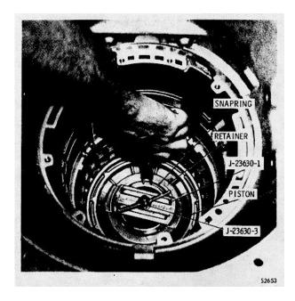
Fig. 7-2. Installing first clutch spring retainer snapring
